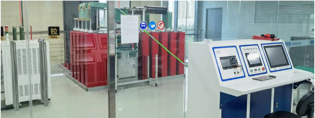
Impulse Current Generator T1 (10/350 \mu s) and T2 ( 8/20 \mu s) test
